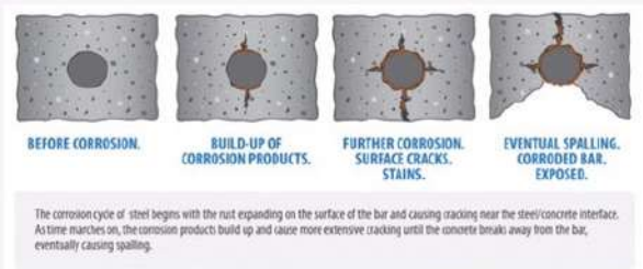
Corrosion cycle of steel reinforcement in concrete
